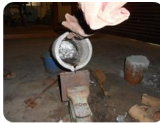
Fig 2. Molten metal poured in pattern
