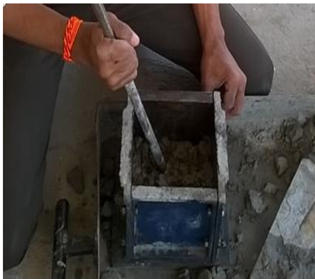
Fig.10 Compacting the concrete in the cube mould (For 150 mm cube at least 25 tamps per layer).
