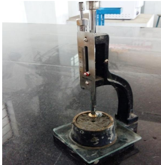
Fig. 4 Final setting time
