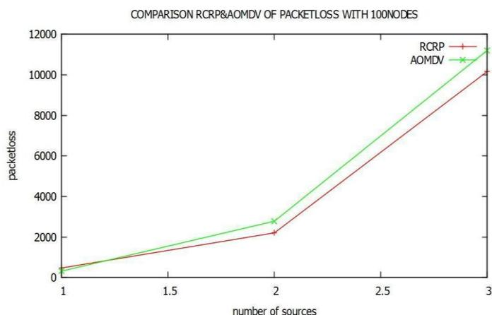
Fig 5: comparison between packet loss of AOMDV and RCRP
