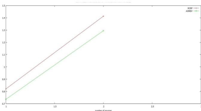
Fig 6: Comparison between delay of AOMDV and RCRP
