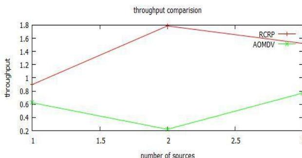
Fig 4: comparisons between the throughput of AOMDV and RCRP
