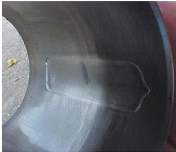
Fig.3.2a circlip explosion
