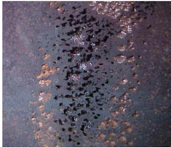
Fig.3.2b cavitation with scales
