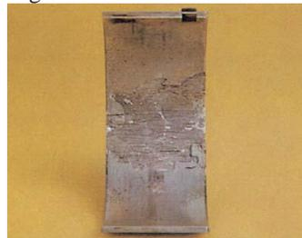
Fig3.3c generalised fatigue
