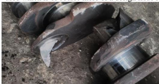
Fig3.4a cracking of crankshaft
