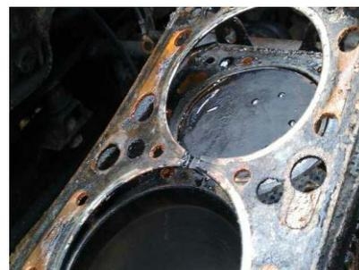
Fig.3.5b blown gasket
