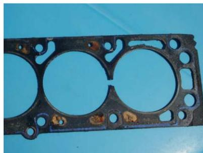
Fig.3.5a worn-out gasket
