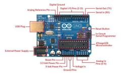
It is an open source single board using microcontroller that is based on ATmega328P. The board is equipped with 6 analog inputs and 14 digital input output pins. It acts as a communication interface which can include USB interface used for programming. It consists of power jack, reset button, flash memory of 32 kb, SRAM and EEPROM, clockspeed (16MHz) and it operates on 7 to 12 V.
