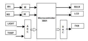
Block diagram depicted mainly focus the major contributing peripherals in making of the entire system and as an example the parameters like light and temperature to be sensed along with the respective sensors are shown.
